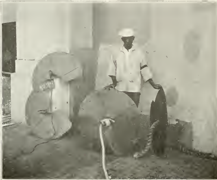
The Panama Canal rat-guard. The strap iron reinforcements give it rigidity and hold it perpendicular to the line. The lashing is a permanent part of the guard and the internal half cones make it fit any line accurately. It is easily and quickly applied and light enough to facilitate handling.
